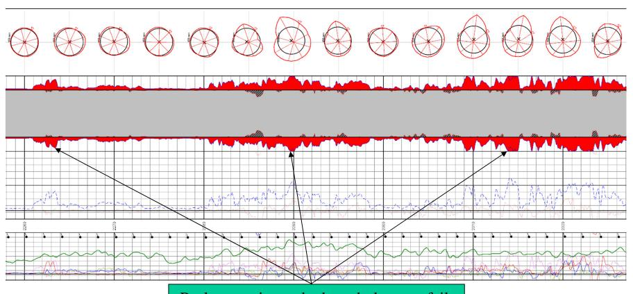
Packers set in washed-out hole may fail, resulting in an ineffective frac operation.
